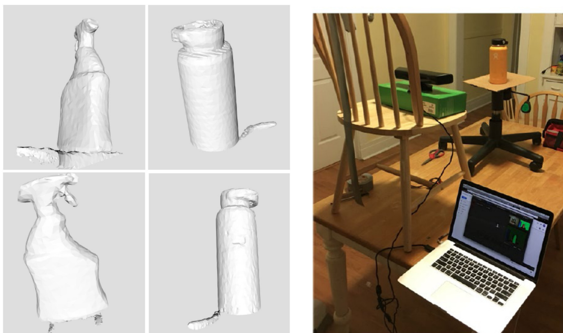
Fig. 3. Scanned objects that students tested with the 3D scanner (left). Students testing a workflow prototype using the XBOX Kinect and a rotating chair (right).
