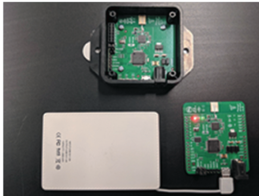
Figure A1. Pozyx anchor (top), Pozyx tag (right) and USB battery pack (left).
